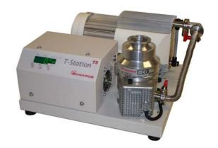
The T-Station comes with our new TAG (Turbo and Active Gauge) controller fitted as standard which enables single button start/stop of the system, the ability to control one of our Active Gauges\*, vent valve\* control and delayed start of the turbopump to either time or pressure if a gauge is fitted, making the T-Station ideal for general laboratory needs.
